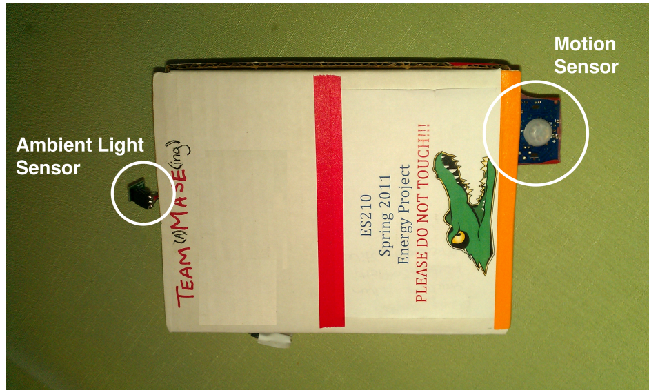
Figure 3. Sensor exterior with motion and light sensors noted.
