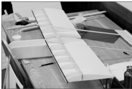
(a) Spar-and-rib wing construction.
