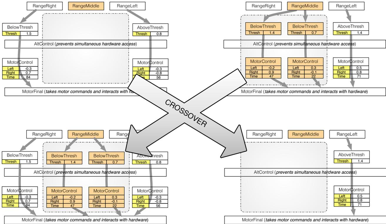
Figure 8: Example of crossover method on two brains, where the chosen swap involves the RangeMiddle sensor
