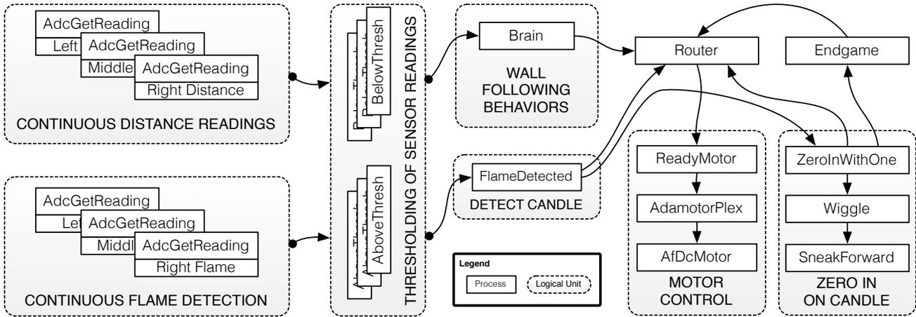
Figure 4: occam-pi process network for physical robot
