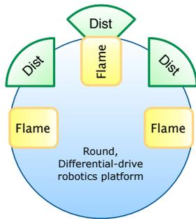
Figure 3: Placement of sensors on the robot
