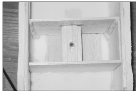
(b) The Gator 's fuselage construction.
